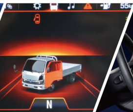
Warning of unclosed door and unremoved key
